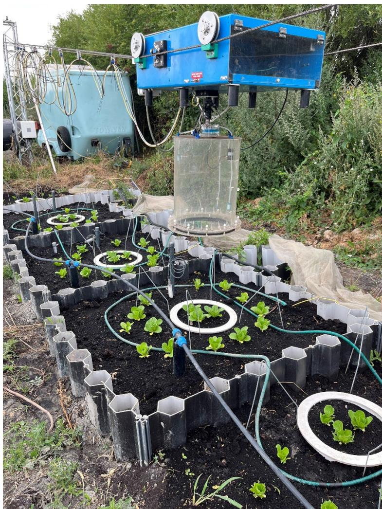
**Figure 5.2.** The Skyline plot-scale irrigation experiment at Rosedene, with recently planted lettuce crop (above) and the plot treatment layout (below)
