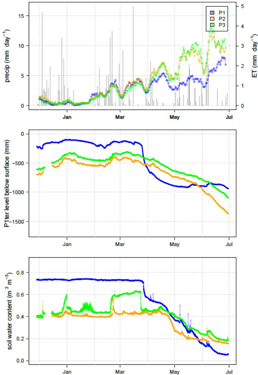
**Figure 5.31.** Precipitation and evapotranspiration (top), water table (middle) and soil moisture content (bottom) for the Pollybell GGR flux towers, December 2021 - June 2022.
