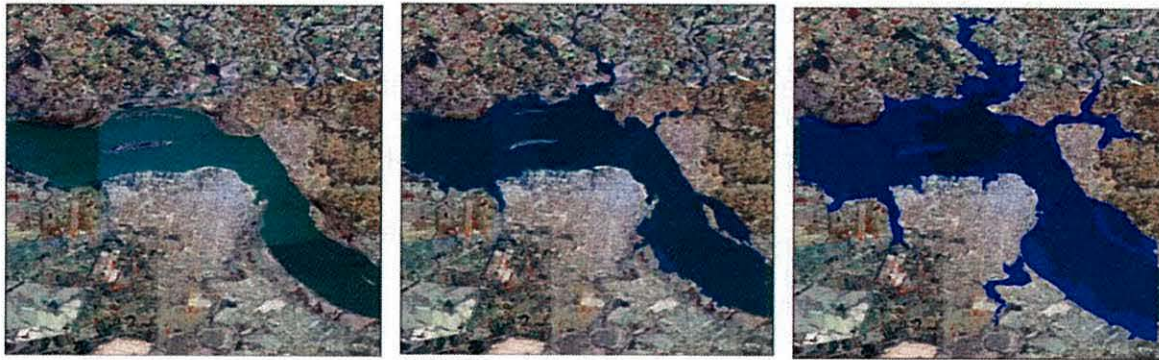
Figure 2. Sequence of approximate flooding of the Yacyreta reservoir in the area of the cities of Encarnacion and Posadas. From left to right: 1) Parana River at original level; 2) current level at 78 m; and 3) expected level of 83 m. Mboi Cae and Quiteria Rivers visible only partially at their junction with the reservoir. Source of Image and drawing: YBE no ref.
