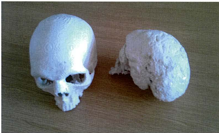
Figure 5.5: Photo of 3D-printed objects based on segmentation data
