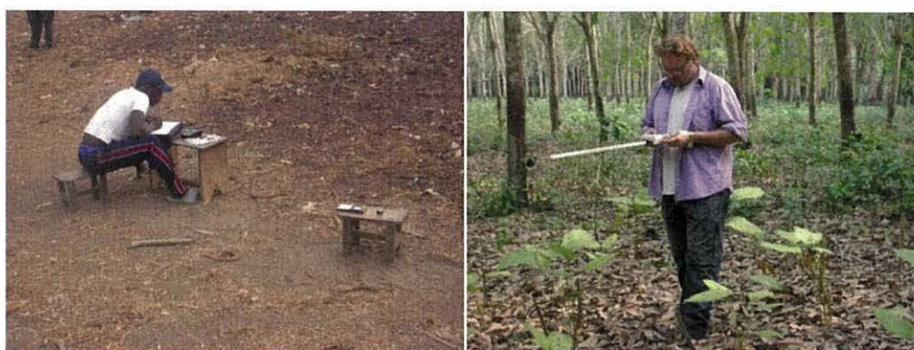
Plate 6.2 Taking measurements of photosynthetically active radiation (PAR) in the open canopy at Missellele Market and under a rubber canopy at Missellele experimental site January 2007 (Photos: Mark Lyonga).
