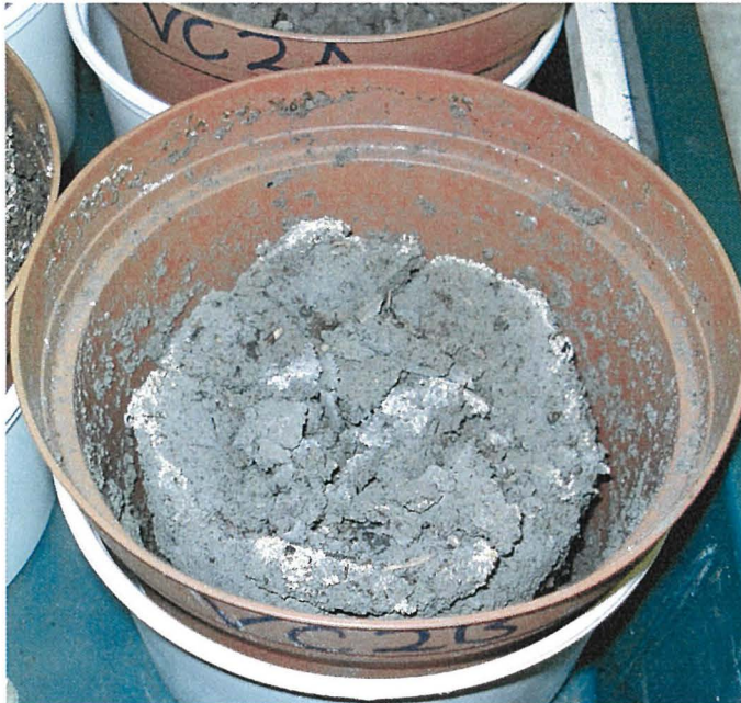
Figure 5.8 Shrinkage in drying vermicompost (V2) made from green waste and paper pulp
