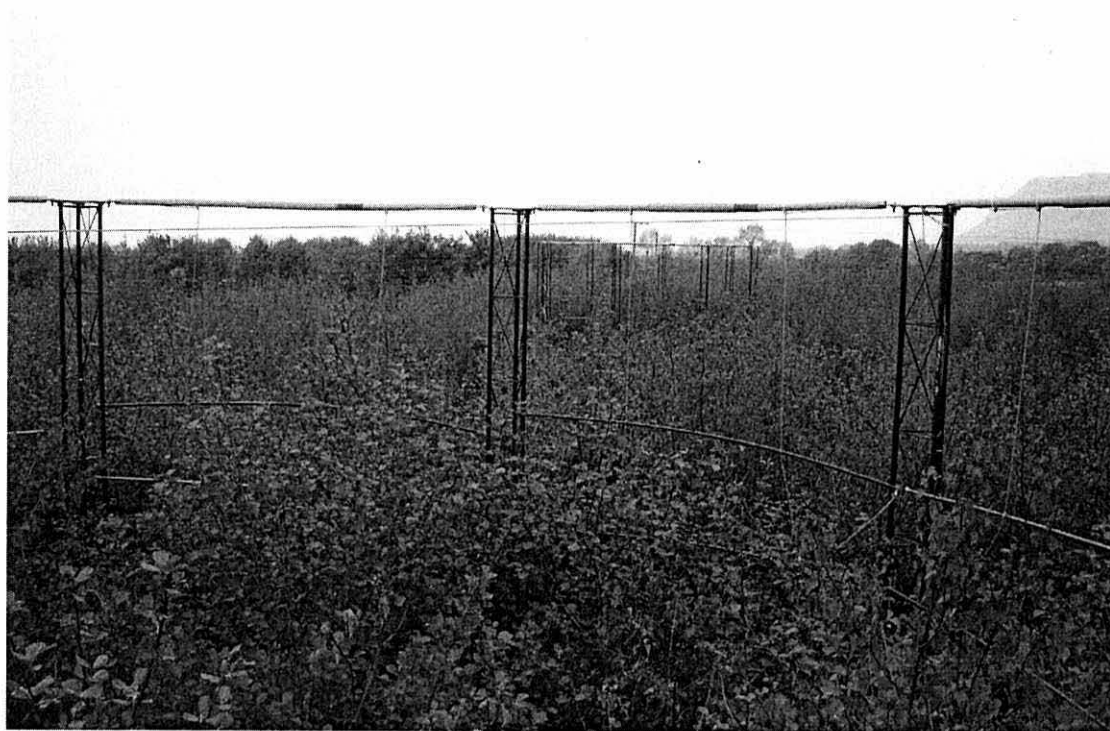
Figure 2.7 The view from the top of plot three during the summer of 2007. Two layers of enrichment pipes can be seen suspended from the infrastructure supplying CO 2 to the middle of the canopy.
