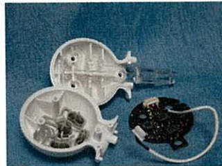
5.Open and remove the circuit board leaving the wire connected
