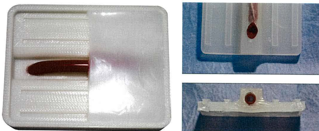
Figure 5-10 Left: The left hand side of the tactile end effectors silicone has been removed to reveal the simulated femoral artery. Right: The profile of the tactile end effector can be seen in the removed silicone section. A simulated femoral artery has been inserted to illustrate its path through the silicone. The ridged profile of the silicone secures it to the plastic base during use.
