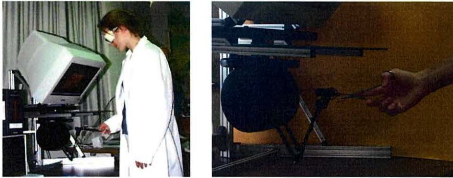
Figure 2-3 Mounting the PHANTOM Premium upside-down for increased range of motion in suturing procedure. Image courtesy of R. Webster.
