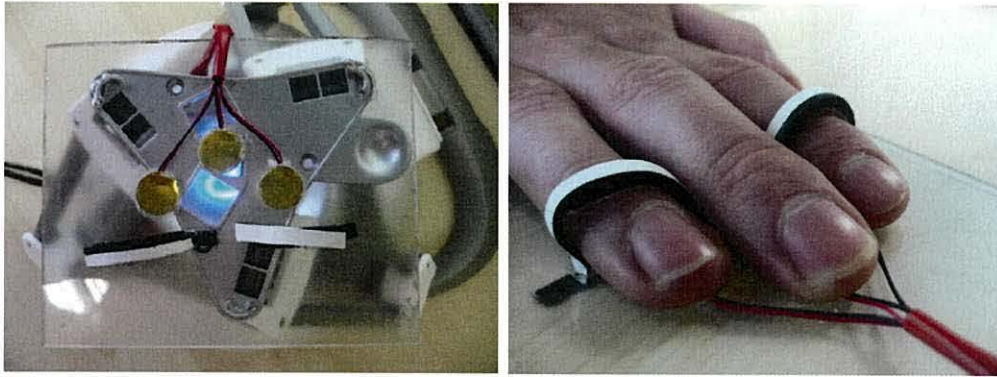
Figure 5-4. Left: Piezoelectric pads mounded onto a customised Falcon end effector. Right: The position of a user's fingertips on top of the modified end effector.
