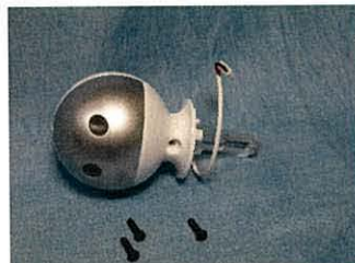
4.Remove the triangular base and another three screws
