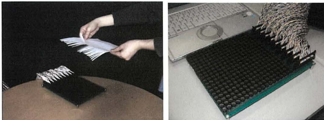
Figure 2-4 A non-contact tactile display based on the radiation pressure of airborne ultrasound provides haptic feedback through air [20].
