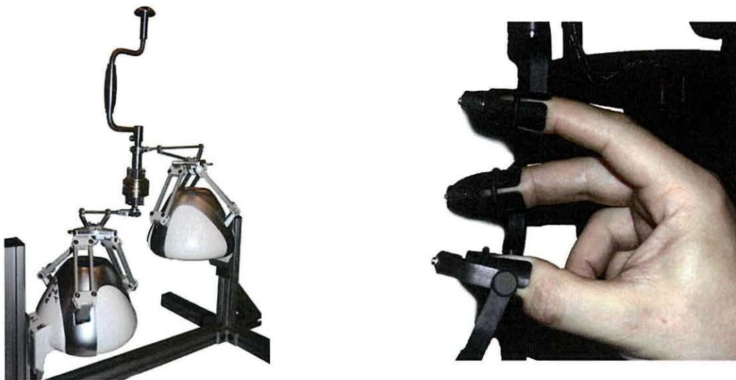
Figure 2-1 Left: Simquest's burr hole drilling simulation hardware. Two 3 force DOF Falcon devices arranged to give 5 force DOF feedback to a single drill handle. Right: McKnight's three fingered haptic setup using three PHANTOM Premium devices to simulate grasping [12].
