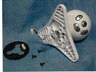
3.Remove the screws and detach the five pin connector labeled P1
