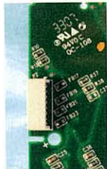
10.The eight pin connector leading from the end effector is labeled P2
