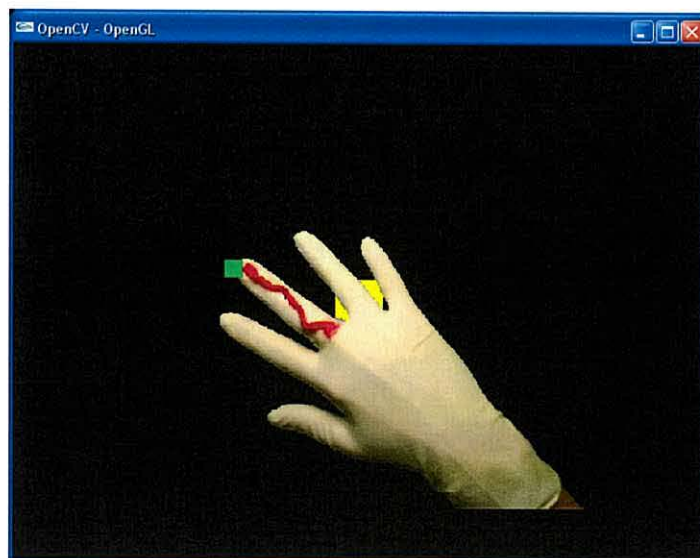
Figure 4-8 Acquisition program. A hand and marker have been extracted. The hand occludes a yellow cube within the scene for testing. The position of a red marker denoted the fingertips position, highlighted here with a green square.
