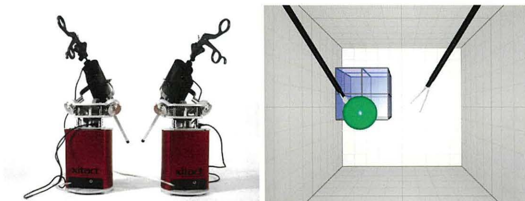
Figure 2-22 Left: The Xitact IHP instrument tracking and haptic hardware for laparoscopy simulation. Right: Core skills training using Mentice's MIST simulator.
