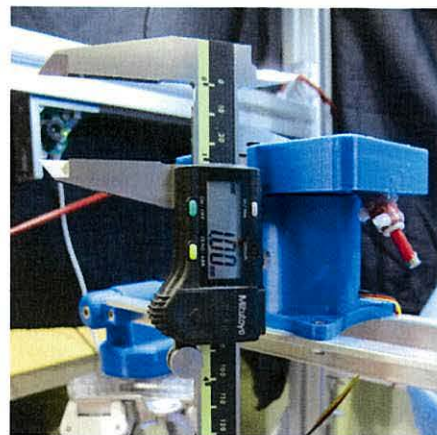
Figure 7-4. Left: A plot for calibration. Comparing the expected device position in red (device reading) with the actual (real world measurement) position in blue. Right: Precise measurement of the end effectors real world position.
