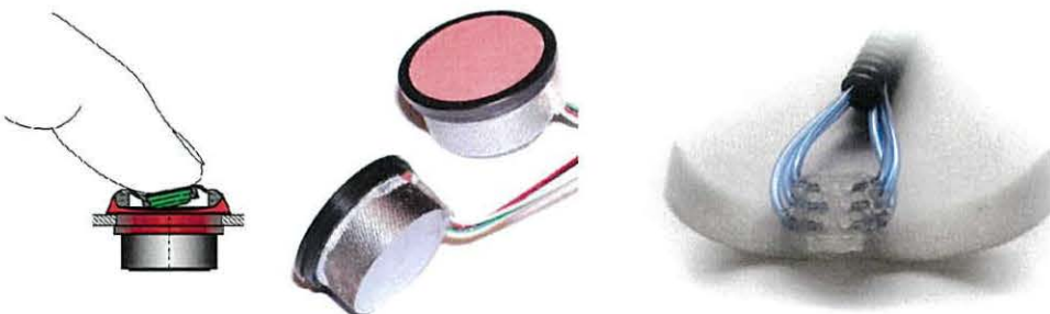
Figure 2-6 Left / centre: Compact tactile interface from CompuTouch AS (Asker, Norway). Right: A pneumatic balloon tactile interface [38].
