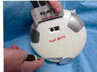
8.The silver dust protectors can be unclipped with a screwdriver
