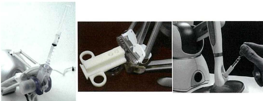
Figure 2-17 Left: One of Novint's custom force feedback grips for needle insertion simulation. Centre: A Falcon used as a master to guide a robotic MRI prostate needle brachytherapy procedure using modified end effector [87]. Right: Chinese acupuncture, original Omni end effector unclipped and a real acupuncture needle is taped to the jack connector [88].
