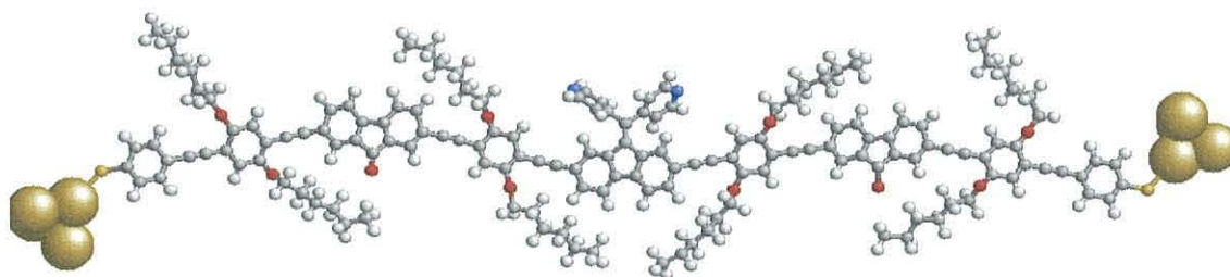
Figure 97 Molecular structure of arylene-ethynylene molecular wire 7 with 7 nm long backbone and thiolated termini.
