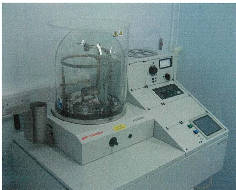
Figure 43 A photograph of a coater unit, Edwards 360A .
