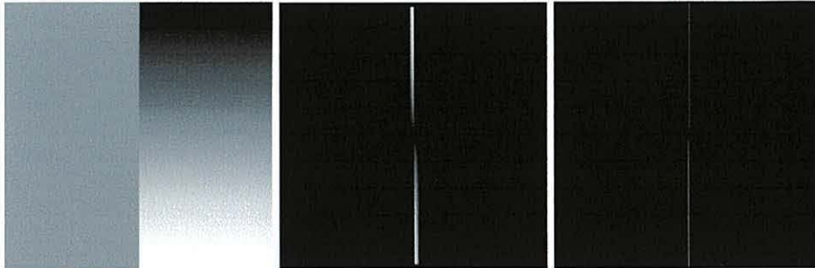
Figure 17: Gradient test image, high-pass result and 2 nd order result
