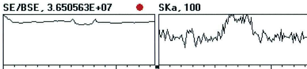
Figure 2.6: [left] A line scan of the sulphur trace in a treated sample of wood & [right] the surface profile of the timber sample.
