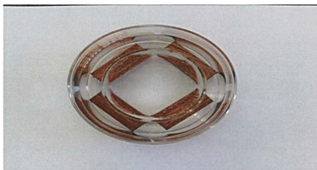
Figure 2.3 The arrangement of wood samples in the circular glass trough
