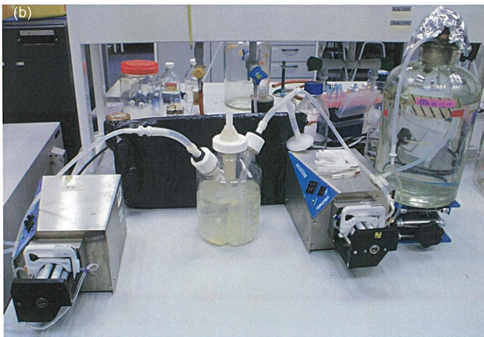
Figure 9.1. (a) Schematic representation of the continuous flow reactor. Black arrows represent media flow and blue arrows represent airflow. (b) Image of the bioreactor, feed and drain vessels, and pumps used to input and to drain the reactor vessel.
