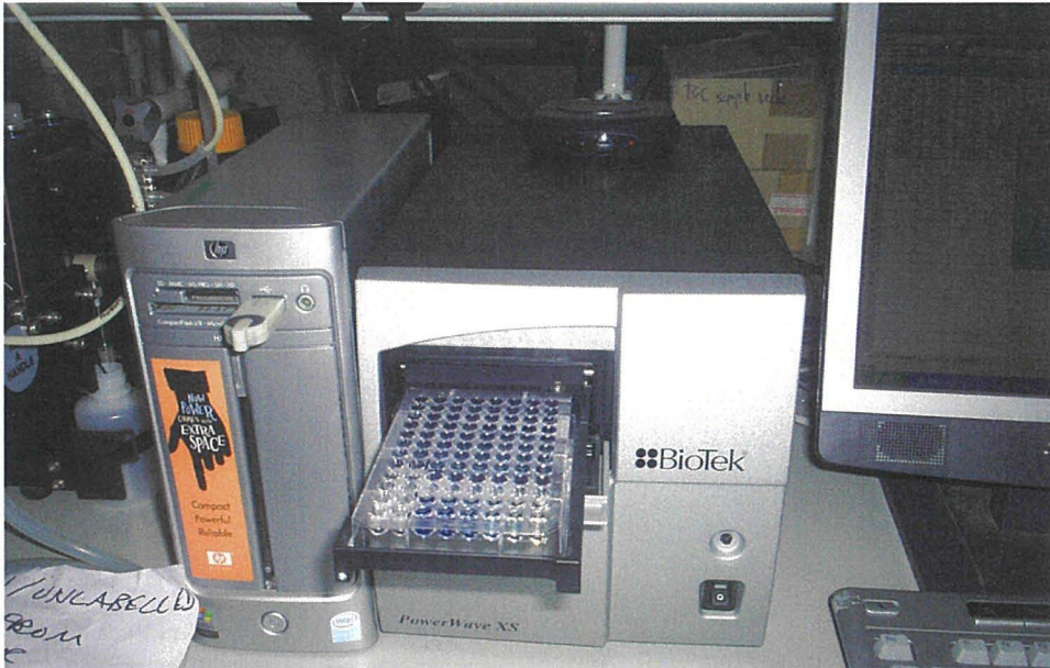
a. Determination of phosphorus content using a spectrophotometer (BioTek, model PowerWave XS)
