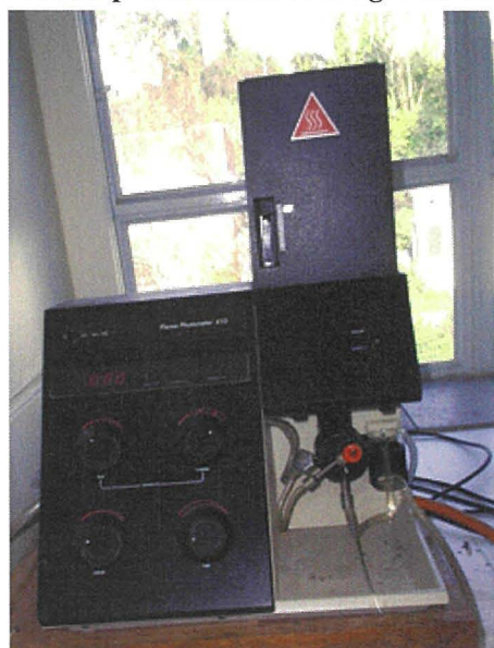
Plate 5.2. The model 410 flame photometer range (Sherwood, Cambridge, UK) used to determine calcium, sodium and potassium in millet grains and taro corms
