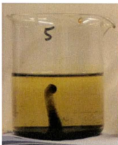
Figure 5.15. Particle shift towards a magnetic force that was held against the beaker wall.
