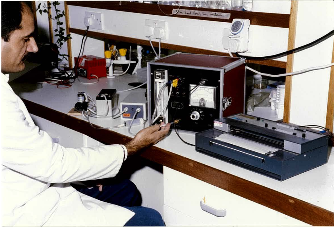
Plate 2.3 Portable gas chromatograph for determination of nitrogen fixation rates.
