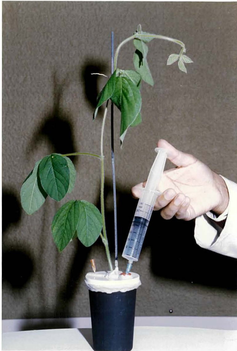
Plate 2.2 The method used to seal and add acetylene into pots.
