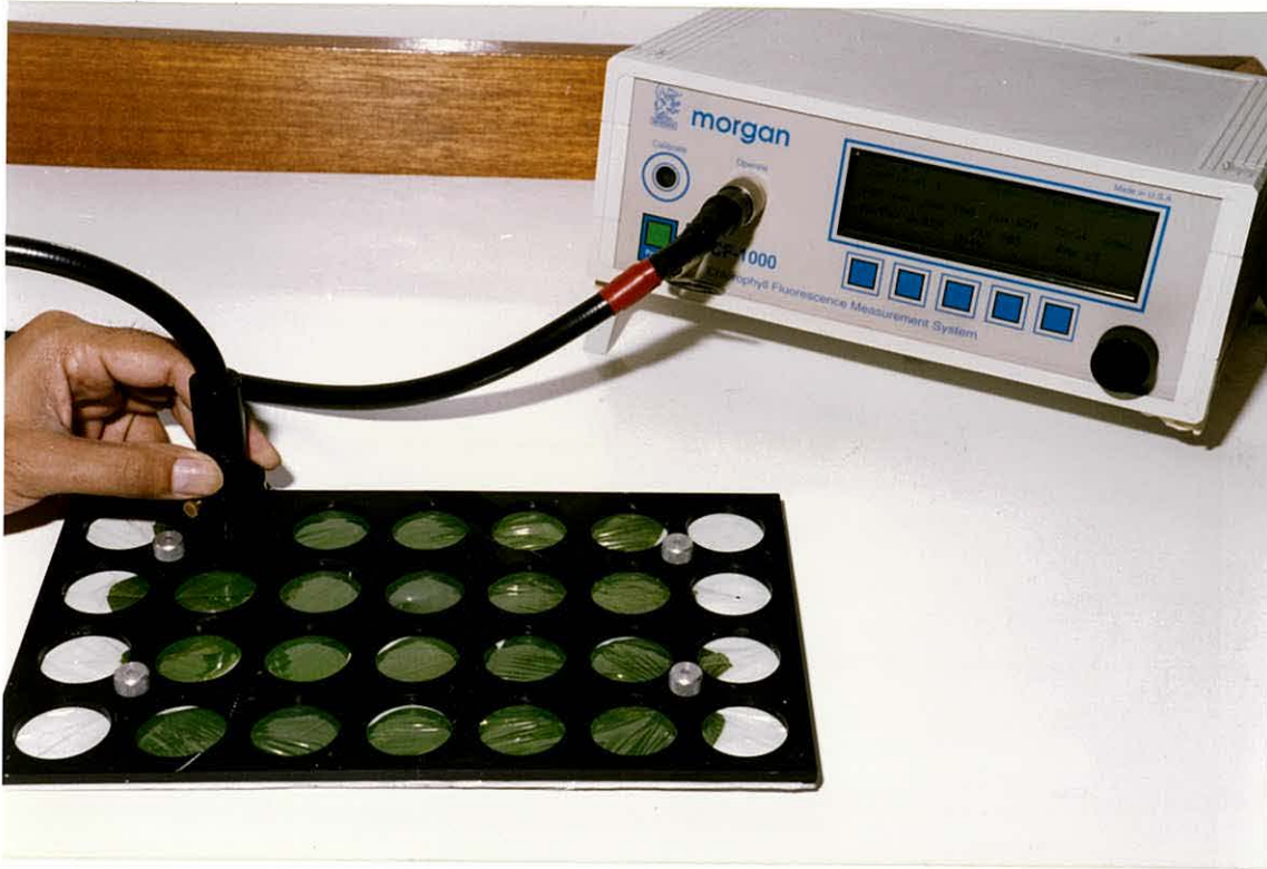
Plate 2.1 The Morgan CF-1000 chlorophyll fluorometer and leaf sample holder.
