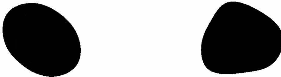
(a) Ellipse: aspect ratio = 1.36, (b) major axis = 138.7 pixels, minor axis = 102.0, angle of major axis to vertical (anti-clockwise) = 0.900 radians (51.6°)
