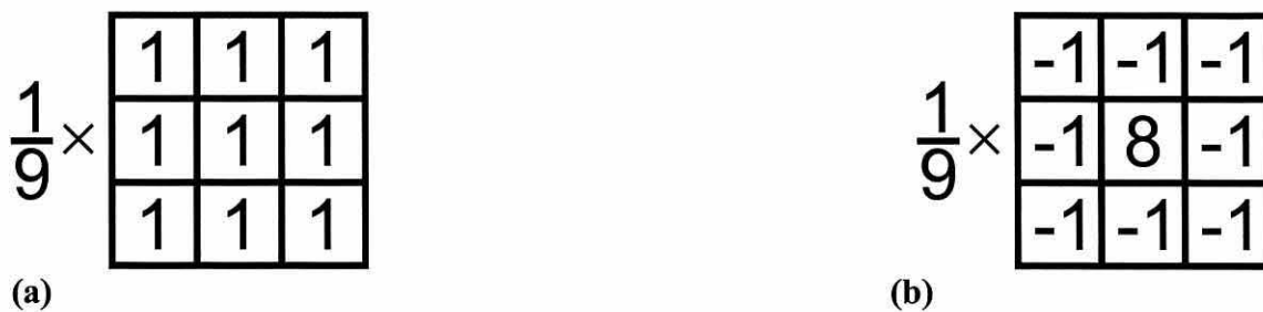
Figure 3-8: Example spatial filtering masks, used in Figure 3-7. (a) Low-pass average filter. (b) High-pass filter.
